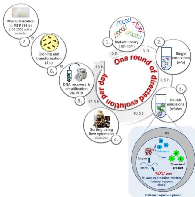
Fig. 1: Principle of InVitroFlow comprising 7 steps. (1.) Mutant library generation using a linear DNA template (approx. 6 h), (2.) entrapment of mutant cellulase library in (w/o) single emulsions within 0.5 h, (3.) cell-free expression of mutant library and generation of (w/o/w) emulsions within 4 h, (4.) sorting of active variants within (w/o/w) emulsions using flow cytometer within 2 h, and (5.) DNA recovery from (w/o/w) emulsions and PCR gene amplification in 3.5 h. A whole round of InVitroFlow (diversity generation, screening by flow cytometry, amplification) can be completed within 16 h. (6.) Cloning and transformation into expression host (2 days), and (7.) screening of up to 2,000 beneficial clones in MTP format and characterization of a few variants (7-12 days).
